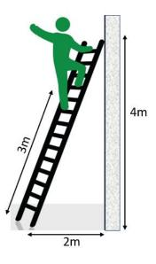
b) Calculate the magnitude *and* direction of the force by the wall on the ladder. Answer in N.
