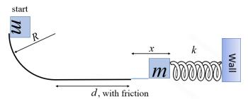
track. The block then compresses the spring to a distance *x* and comes to a momentary stop, on a frictionless surface again. The spring k=100N/m.
